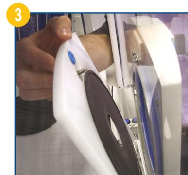
3 Tilt the carrier down to its lowest position, parallel to the workstation floor.
