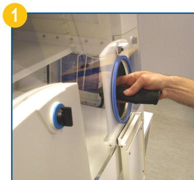
1 Roll a replacement membrane and insert into the workstation through the membrane that is not being replaced.
