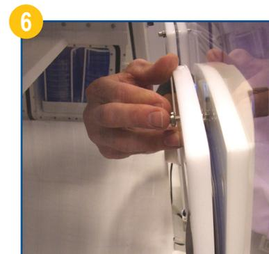
6 Raise the membrane carrier back into position. Tighten the screw until the carrier is firmly in place.
